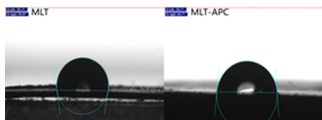
Figure 8. Contact angle images of MLT and MLT-APC.
